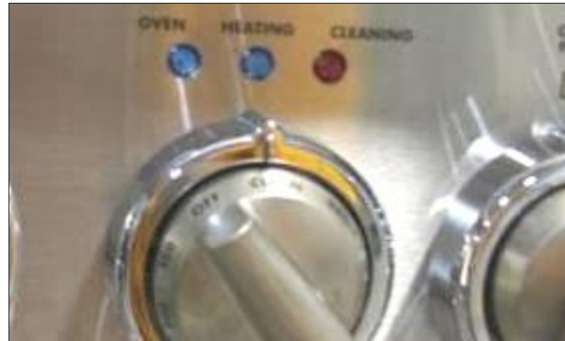
Figure 16: Three Horizontal LED Indicators (Only Blue LEDs Blink)
