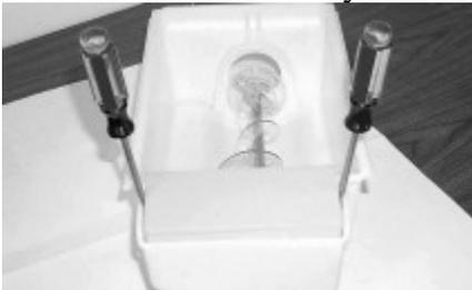
8. Slide the back cover off the auger. The back cover must be replaced because of tabs broken off for disassembly.
