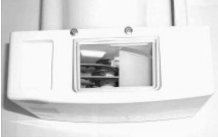
3. Turn over the ice bucket and ice dispenser cover. Remove the Phillips screw.
