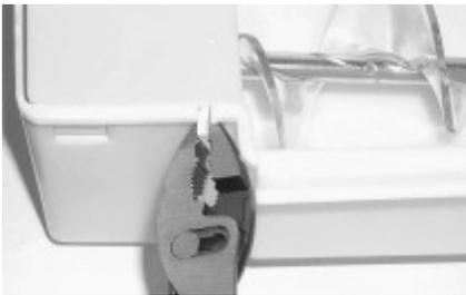
6. Using a pair of pliers, break the tabs off the back cover.
