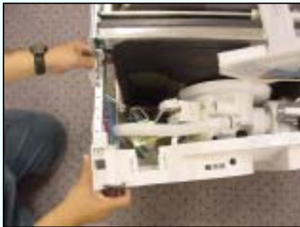
Carefully pull base away from tank & sump
