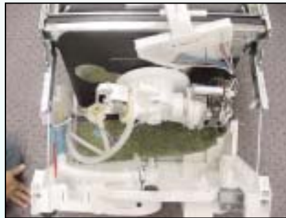
Carefully pull base away from tank & sump
