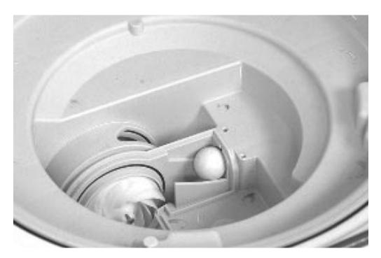
When the pump starts, the force of the water pushes the ball to block the opening to the upper arm delivery tube.
