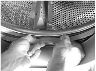
5. Using your thumb, start on the other side of the top tab and force the bellows on in the other direction. Again about one third of the way around stop and seat the bellows onto the tub lip. Then force the remaining bellows on with your thumb and seat it. 6. To install the spring, fold the front of the bellows back into the tub.
