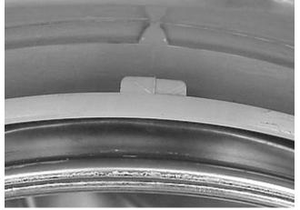
and a slot in the groove and an arrow at the top of the bellows.
