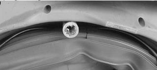
8. Pull the spring with one hand while working it into the grove with the other.
