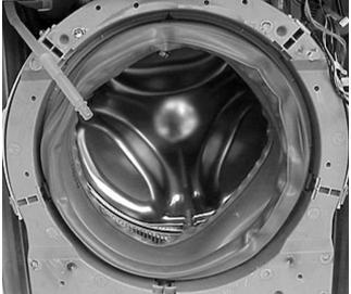
7. Place the spring in the groove at the top of the bellows and wedge a round object, about 3/4 " in diameter, between the weight ring and the bellows to hold the spring in the groove.
