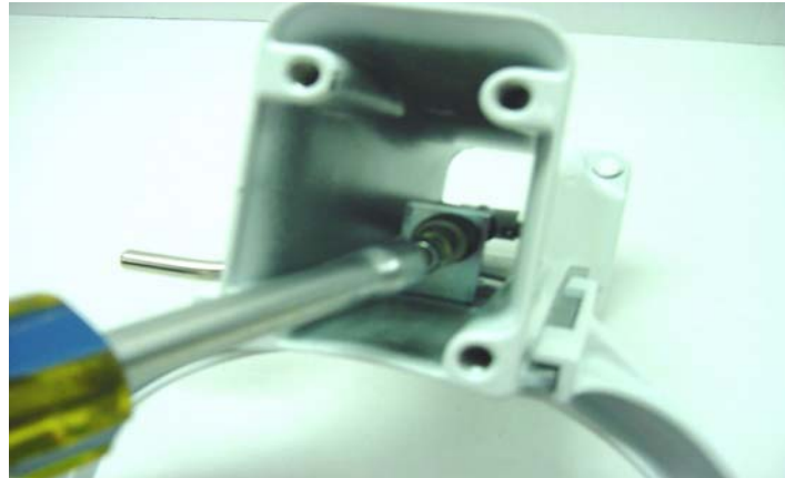
Fig. 92 Check the castle nut for proper tension on the bowl lift bracket.
