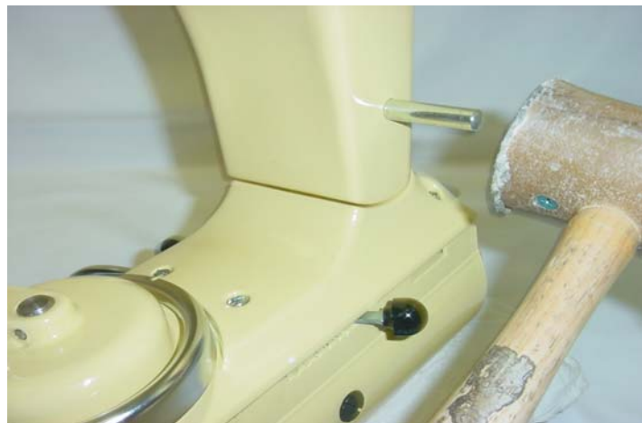
Fig. 73 Use a rubber or rawhide mallet to tap the hinge pin into the pedestal.
