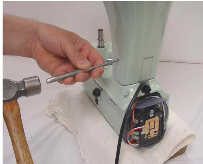
Fig. 4 A drift punch and hammer is used to drive out the hinge pin.
