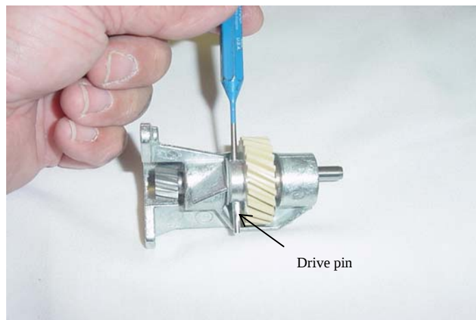
Fig. 57 The drive pin must be removed to change the gears.
