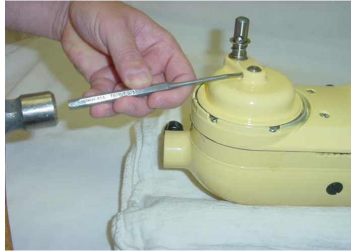
Fig. 68 Carefully drive the groove pin into the shaft of the planetary.
