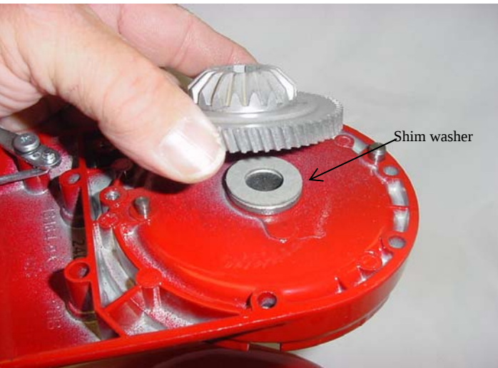
Fig. 55 Bevel center gear being lifted for inspection.
