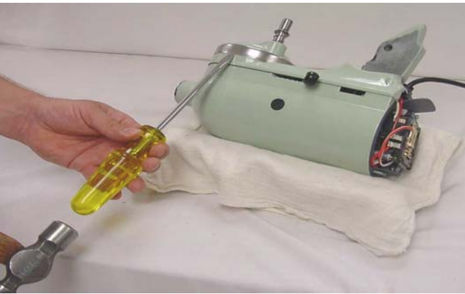
Fig. 5 The Drip Cup fits tightly and must be started off by tapping it.
