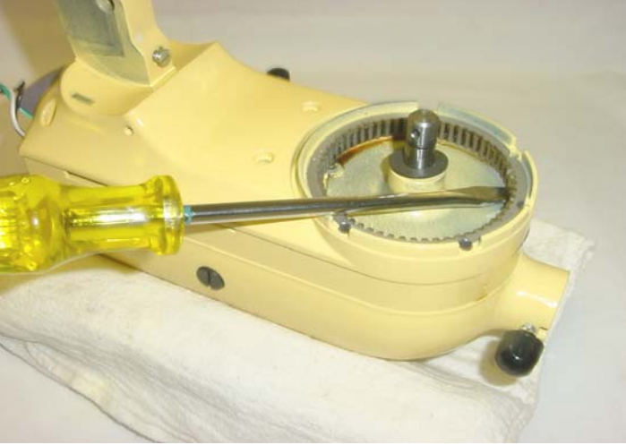
Fig. 61 Internal gear can be pried from the bottom cover and replaced if necessary.
