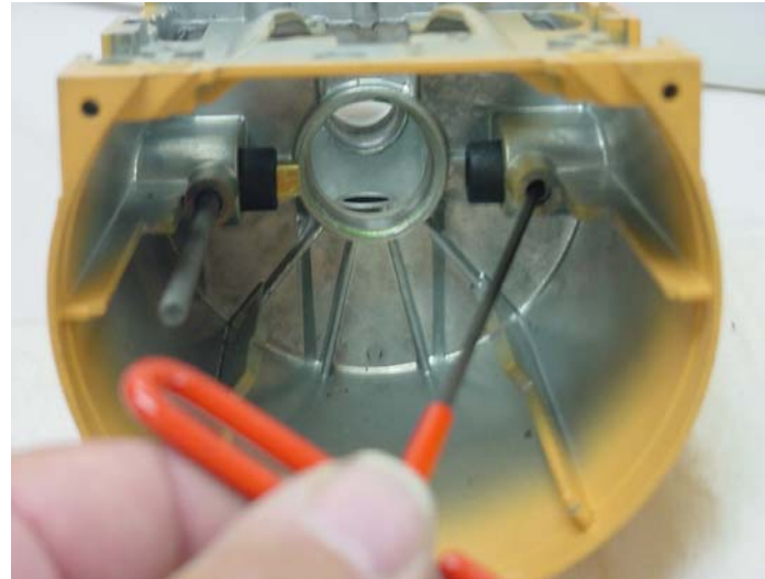
Fig. 31 Wire orientation inside the gearcase-motor housing
