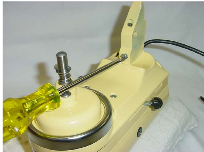
Fig. 69 The adjusting screw has a nylon insert and should not be loose in the threads.
