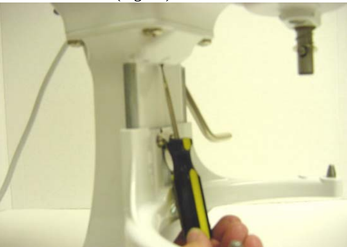
Fig. 97 Adjusting the beater to bowl height using the adjusting screw.
