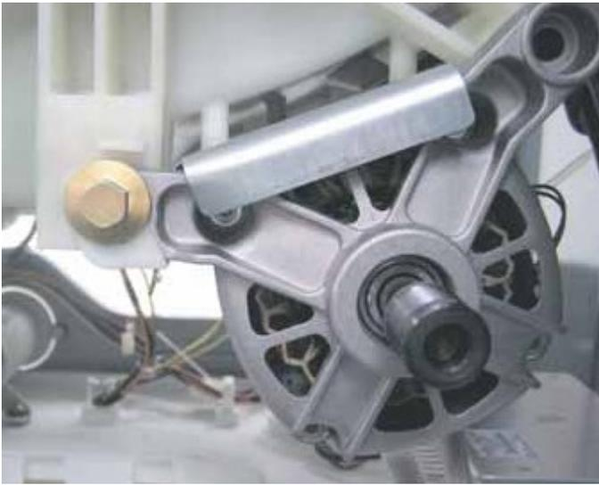
**Note:** The threaded plate can fall out of the recessed slot in the motor mount. Ensure this plate is reinserted in the slot upon reassembly.
