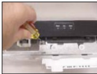
Removing fascia screws
