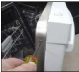
Removing door screws
