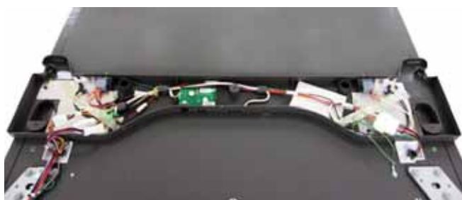
Hinge Cover Service Position
