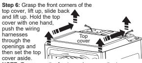
**NOTE:** To remove the front panel, remove the two screws from the top front panel corners, and disconnect all of the connectors and the water line. Set the front panel aside.
