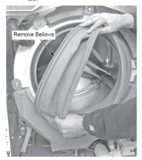
**REASSEMBLY NOTE:** When you reinstall the bellows, be sure to position the "weep holes" at the bottom, as shown below.
