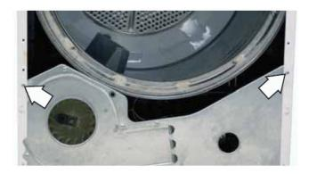
3. Grasp the drum firmly at the 11 o'clock and 1 o'clock positions. Brace the bottom of the drum against your leg and maneuver the drum out of the cabinet.
