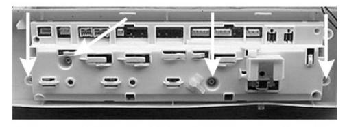
Release the locking tabs and lift the control from the console.
