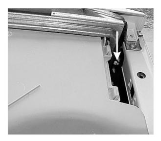
5. Release the (3) locking tabs at top rear edge of the console and roll the console forward.
