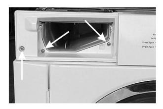
4. Release the tab that is spread open by the left hand screw as view from the front.
