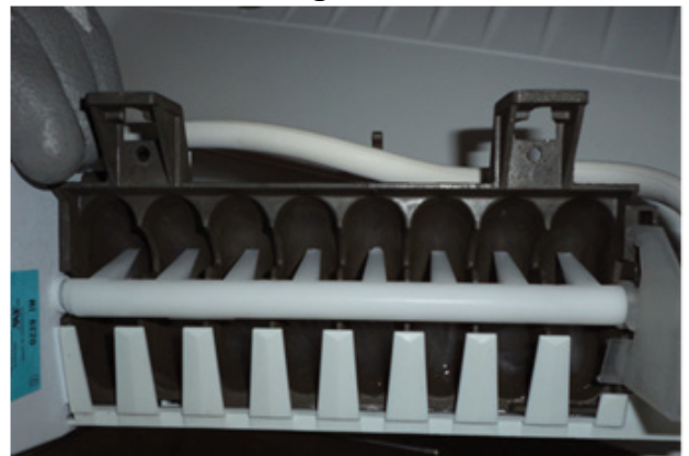
IM ejector fingers at 7 o'clock position (viewed from front of IM)
