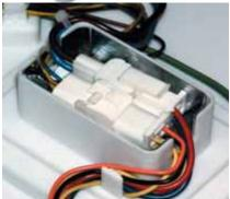
Disconnect the motor wire harness.
