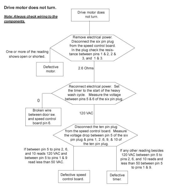
NOTE: If the drive motor windings check open or shorted check the fuse on the speed control board. If the fuse is open, replace the motor and speed control board.
