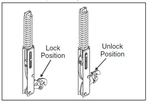
3. Reverse procedure to reinstall oven door.
