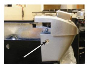
• Remove the two screws under the console.
