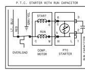
\*CAPACITOR IS ONLY USED WITH SOME P.T.C. MODELS
