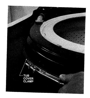
Note: When assembling the tub cover and gasket, be sure all sides of the gasket are clean. Be sure that the triangular rubber gasket is not twisted or outside the clamp. All sides of the gasket are equal and it will make no difference which side is placed against the outer tub and tub cover. Wet the gasket before repositioning between the tub cover and outer tub to aid in the positioning of the top cover.
