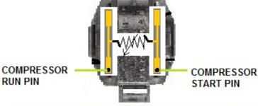
SUPPLY VOLTAGE IS CONNECTED AT THE OVERLOAD (COMMON COMPRESSOR PIN) AND THE RUN TERMINAL ON THE RELAY (COMPRESSOR RUN PIN)
