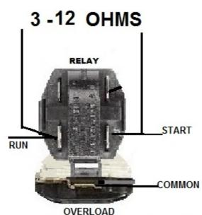
TERMINALS ON THE RIGHT SIDE OF THE RELAY ARE CONNECTED TOGETHER AND THE ONES ON THE LEFT SIDE ARE CONNECTED TOGETHER
