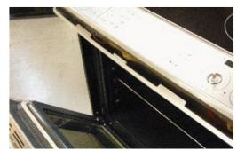
• Remove the screw on both side of the console.
