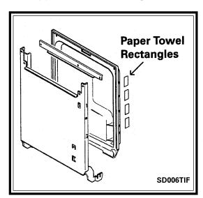
however that may not be where the water is originating from. To determine the origin, a simple paper towel test can be conducted. To perform this test, cut a piece of paper towel into sixteen (16)
