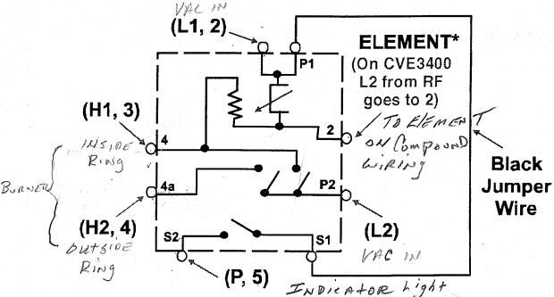
\*On units with a compound connection, the two red wires must be separated. Locate the right front switch connection (L2). The red wire routed from the right rear element/switch will remain, but the red wire routed from the left rear element/switch must be disconnected, reterminated and connected to position 2 on the new dual switch.
