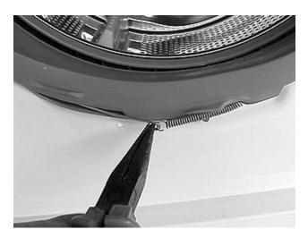
3. Pull the bellows off of the lip of the front panel.
