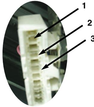
Normal resistance is approximately  $3.0\Omega$  between any 2 pins (1,2,2 or 3) on motor connector.
