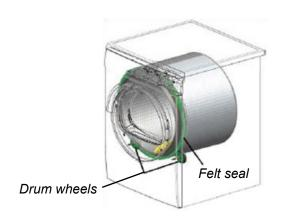
If the seal doesn't fit snugly against the drum, it can be reshaped. After the seal is attached to the drum, wet the seal thoroughly using a spray bottle. Shape the seal toward the drum and run the dryer 20 minutes on a heated timed dry setting. Since felt shrinks when dried rapidly, the seal will shrink to the drum and fit it snugly.
