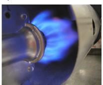
The gas dryer burner circuit runs through the motor & Hi-limit. The connection through the motor cuts out the burner if the motor isn't running.
