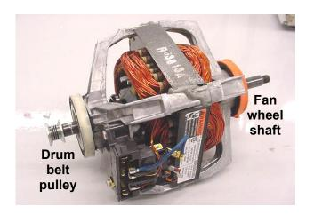
Motor is rated 120 VAC, 60 Hz, 1/3 HP (248.5 W), 5.0 A, 1725 RPM, 40°C ambient, class B insulation. It drives the fan (in front) and drum (in rear, using pulley shown).
