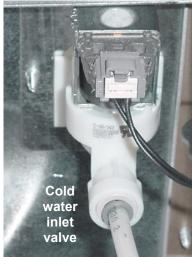
A 90° elbow connects the hose to the nozzle (through a hex adapter). It can be accessed by removing the front panel.
