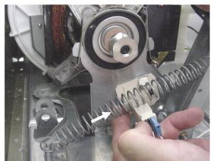
Push <u>left</u> plunger (toward right) to reset broken belt switch whenever drum or belt has been removed for <u>any</u> repair.
