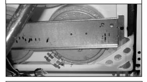
**4.** Remove the mounting screw that secures the element support channel to the cooktop.
