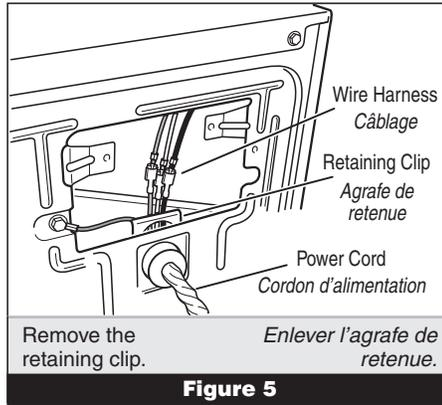
Remove the retaining clip. Enlever l'agrafe de retenue.
