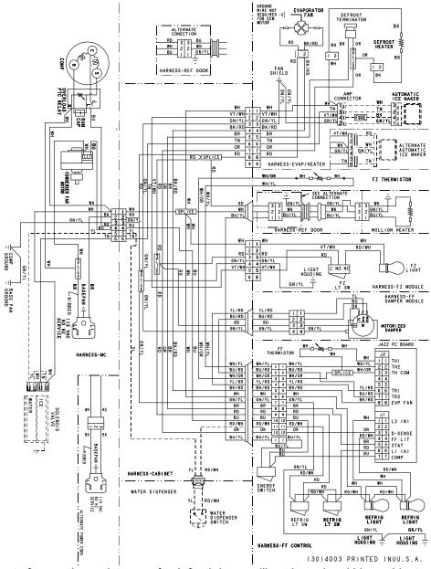
**Note:** In the event of excessive moisture on fresh food door mullion, the red and blue cabinet wires to door harness can be reversed to power fresh food door mullion heater continuously. This will help to reduce moisture on fresh food door mullion. See wiring alternate above for wiring in mullion heater for continuous operation. When powered continuously Energy Switch is no longer in heater circuit.
