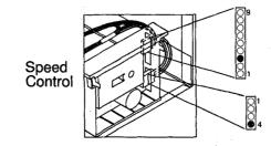
Remove electrical power from the washer. With an ohmmeter check the resistance between pins 1 & 3 of the four pin plug. If the meter reads about 6 ohms replace the speed control board.
