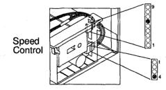
Measure the voltage drop between pin 3 of the nine pin plug and pin 4 of the four pin plug. (Leave meter connected for more than 4 seconds) If the meter reads 0 check timer contact 24 to 24B. If the meter reads 120VAC go to step 6.
